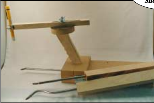
Left: Don Johnson – The laser guided, stabilized, long boring bar that Don built to fit his mini-lathe
