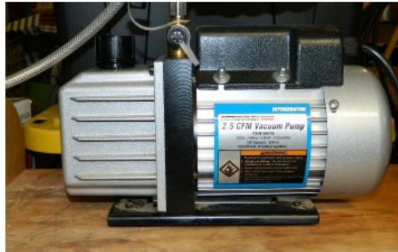
Figure 1 Vacuum pump used for stabilizing projects.
