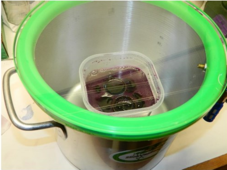
Figure 4 Blanks submerged in dyed stabilizing solution and under vacuum. Note the high-tech weights to keep the blanks submerged. Bubbles emerging from the solution is the air being extracted from the wood.
