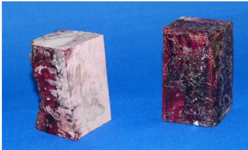
Figure 5 Stabilized and dyed bottle stopper blanks
