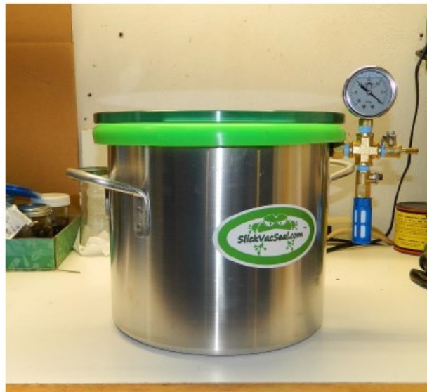
Figure 2 Three-gallon vacuum chamber, gauge, valves and filter
